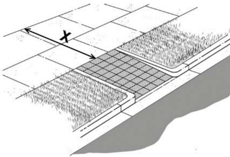
When pedestrians are not required to walk across the ramp, such as where there is a non-walking surface (grass, for example) or obstructions on both sides of a curb ramp, curb ramps are allowed to have **returned curbs**. A curb ramp with returned curbs is required to have a landing with maneuvering space at the top of the ramp
