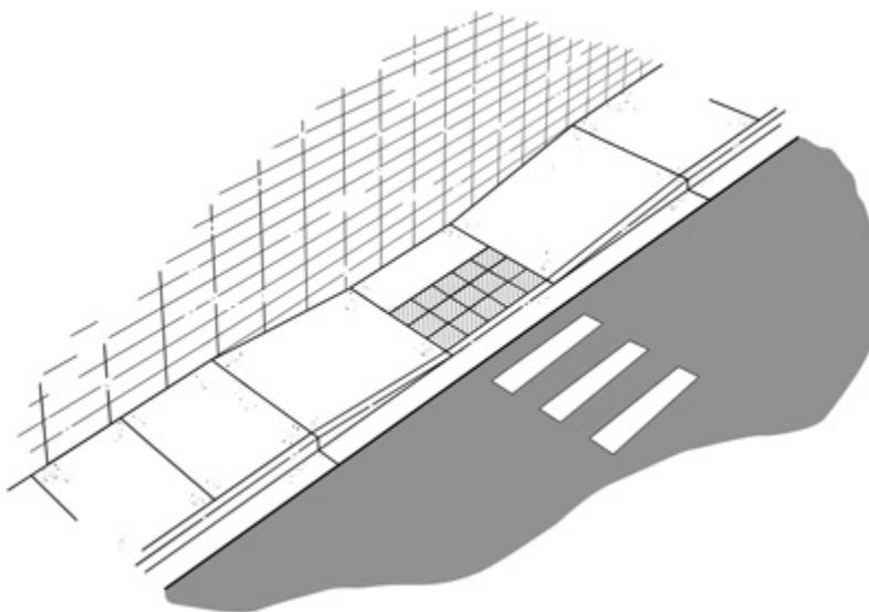
A **parallel curb ramp** consists of two ramps joined in the middle by a landing that is level with the roadway. Parallel curb ramps run parallel to the curb and usually take up the whole width of the sidewalk.
