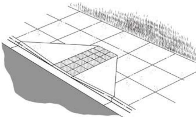
Under the ADA Standards, curb ramps are required to have detectable warnings that extend the full width and depth of the curb ramp.<sup>14</sup> An example of a perpendicular curb ramp that complies with this requirement can be seen to the left.
